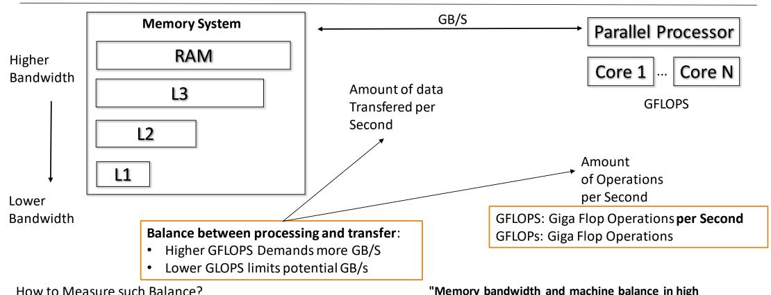
**Arithmetic Intensity (AI)**: Ratio between work performed and data transfered: Flop/Byte.
