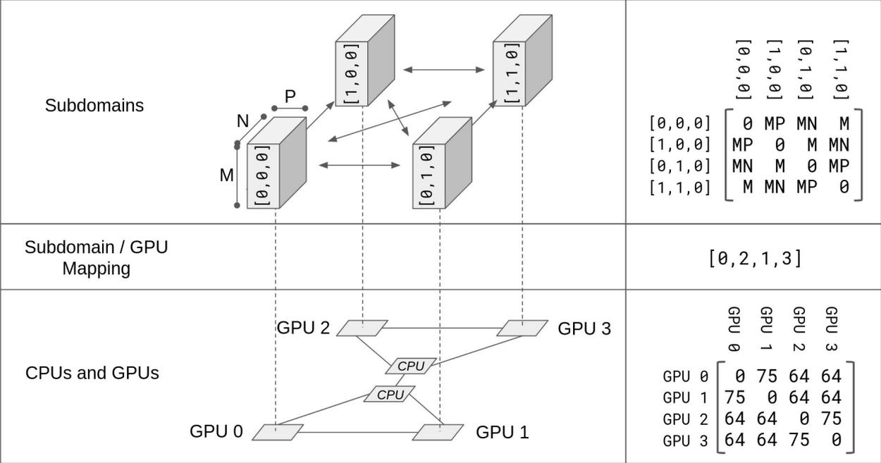
How to place subdomains on GPUs to maximize bandwidth utilization?
